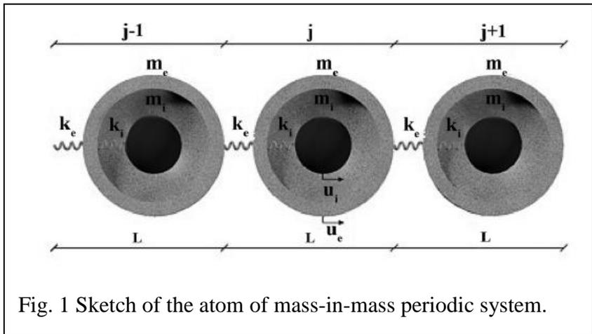
Fig. 1 Sketch of the atom of mass-in-mass periodic system.
